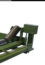
The TAB scale model was designed for weighing bulk products in the extractive, mineral, cement, fertilizer or phosphates production, agri-industry, sugar refinery, timber, recycling industry market sectors and other activities using belt conveyors.
